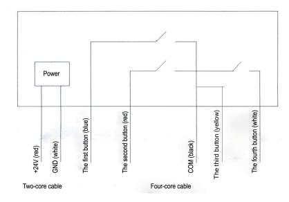
Reference to the following **wiring diagram**: 4 channel relay correspond the first, the second and the fourth button of the remote.
