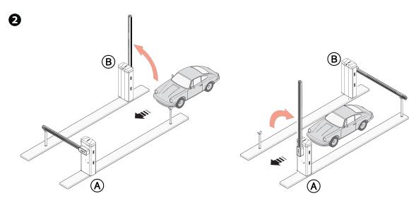
3 OPEN-CLOSE command (2-7) on barrier A or B for emergency opening
