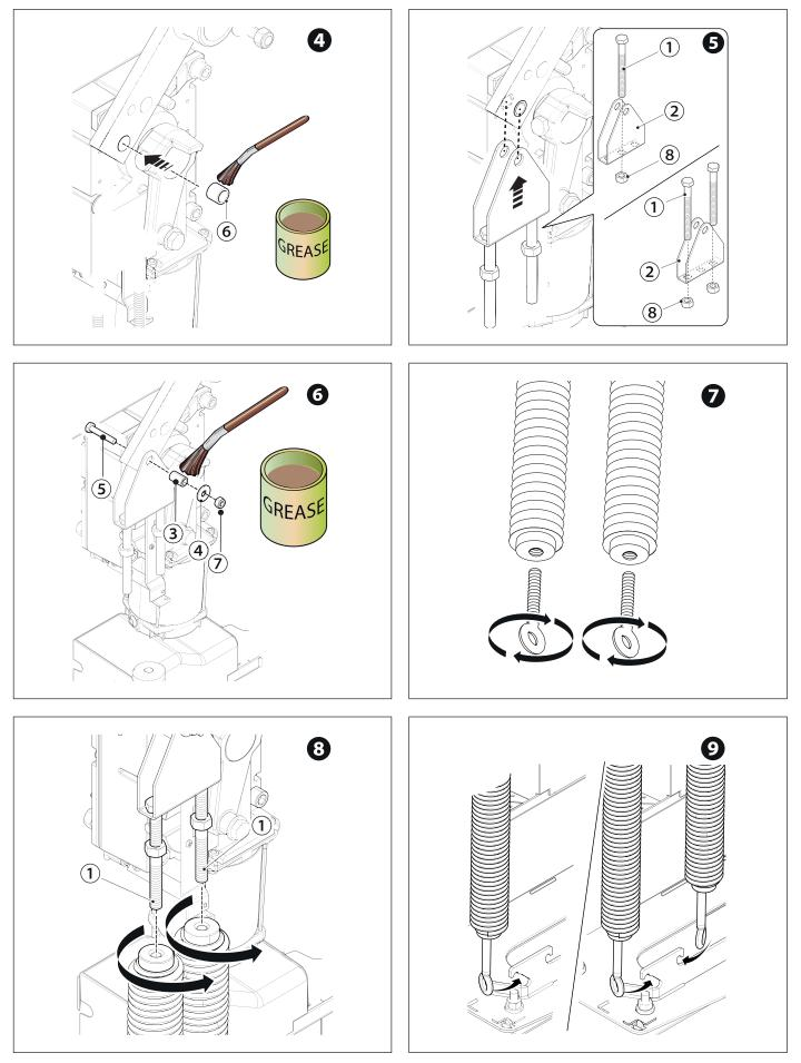
Lubricate the spring when it is fully extended.
