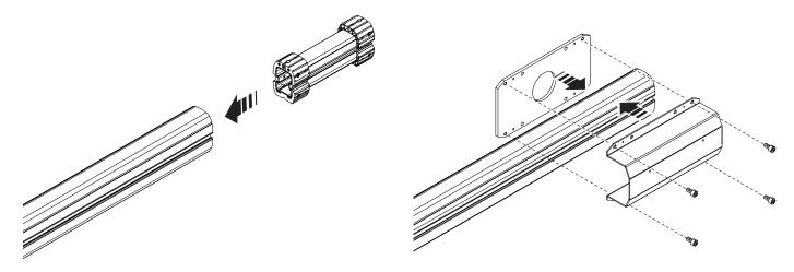
Fix the boom to the anchoring plate.
