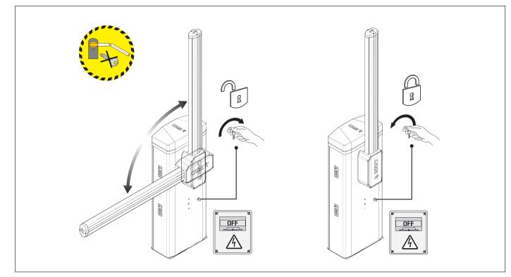
⚠ The balance springs must not be tensioned (boom vertical) when performing maintenance on the barrier.
