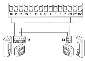
**DXR - DLX photocells** Connection with safety test
