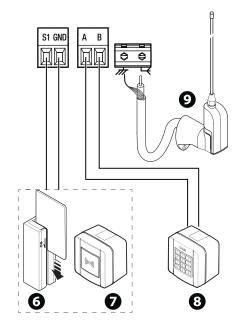
The CXN CAME system is a two-wire non-polarised communication BUS which allows you to connect up all compatible CAME devices.
